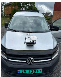
Figure 5. RoadSens platform attached to a passenger car.
