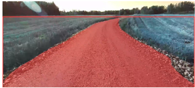
Figure 6. RoadSens footage with the masked roadway. Image: Mostafa Hoseini
