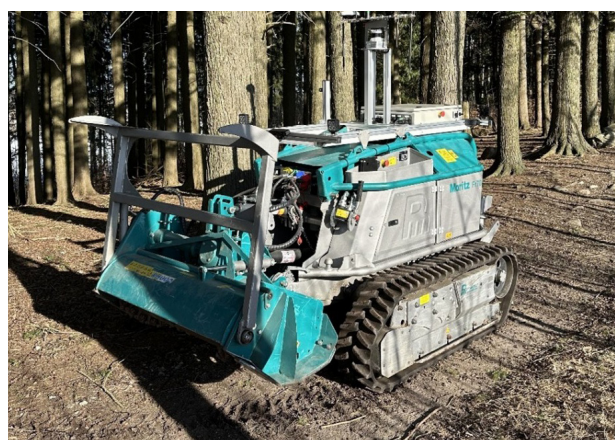
Figure 8. The mini felling tractor Moritz Fr70 upgraded with different sensors, including LiDAR. Image: Csongor M. Horváth, Steffan Lloyd, NIBIO
