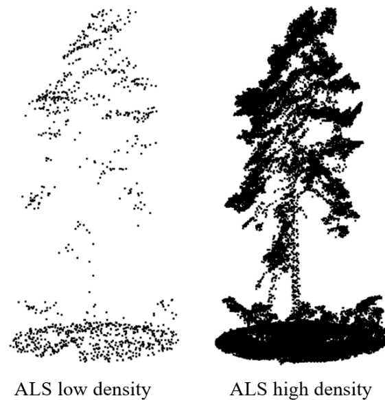
Figure 6. Pine left as retention tree in a harvested stand, illustrated with ALS at low (~2 pulses/m 2 ) and high (~200 pulses/m 2 ) pulse densities. Image: Marie-Claude Jutras-Perreault, NMBU
