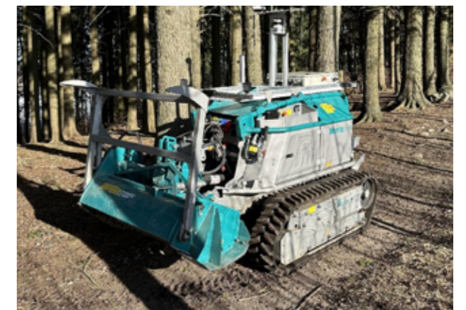
Figure 8. The mini felling tractor Moritz Fr70 upgraded with different sensors, including LiDAR. Image: Csongor M. Horváth, Steffan Lloyd, NIBIO
