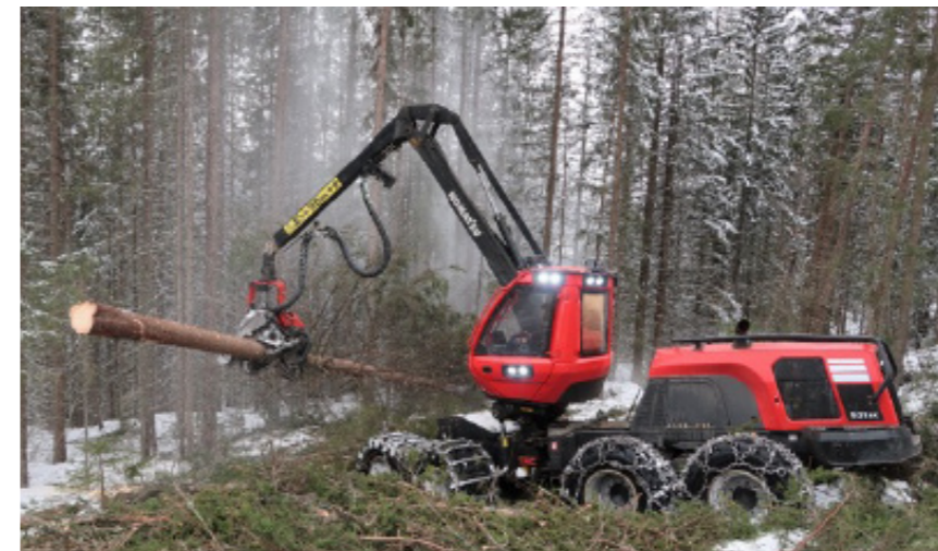
Figure 2. The prototype system on a Komatsu 931XC is based on a number of sensors in the crane that provide information about where the crane tip is at any time. Image: Lennart Noordermeer, NMBU
