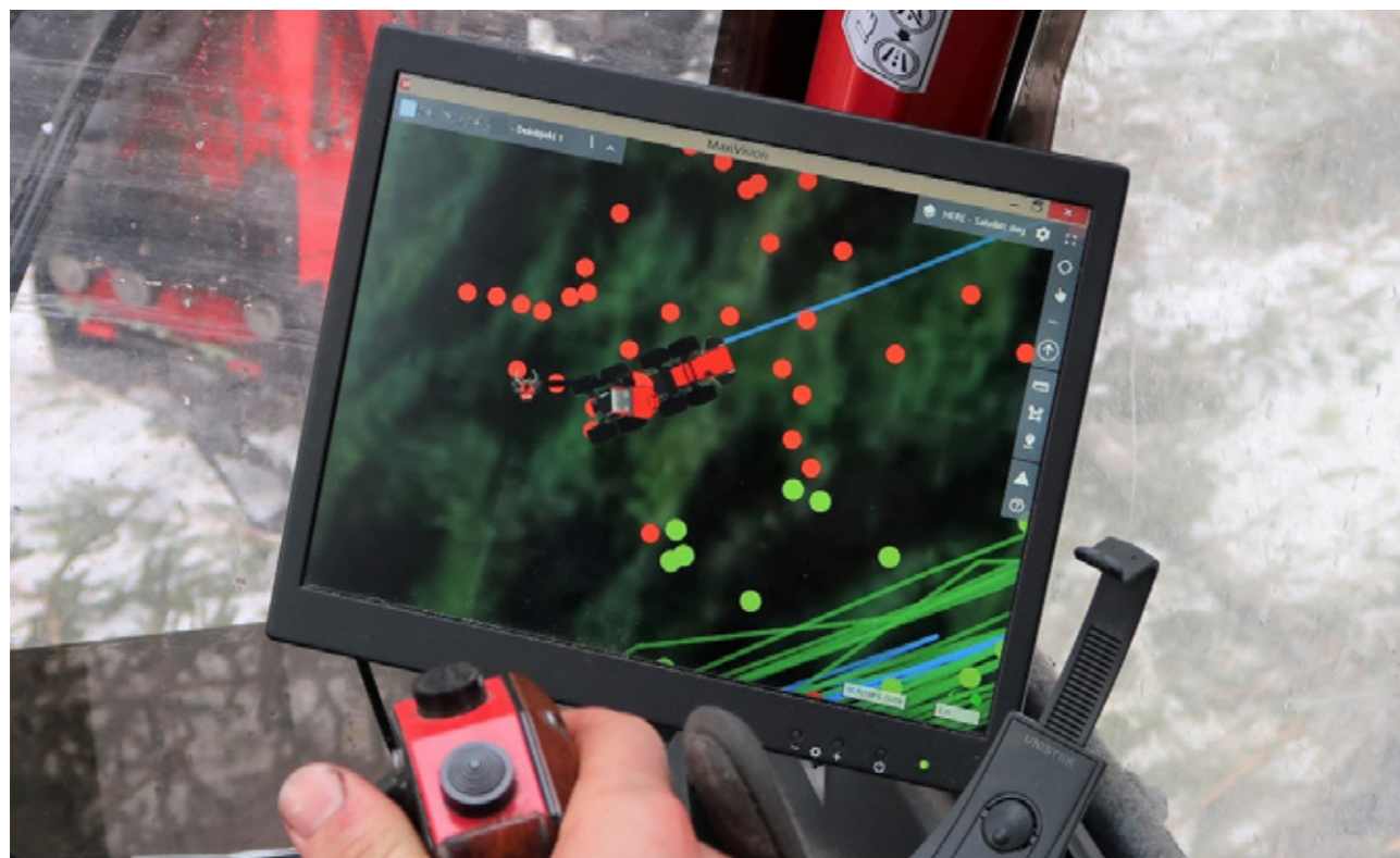
Figure 1. The computer screen shows, among other things, the positions of the harvester, the harvesting unit and felled trees. Image: Lennart Noordermeer, NMBU
